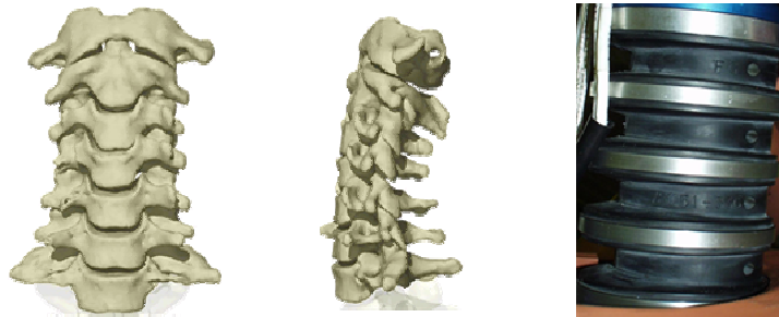
Figure 16: Anterior and Lateral Views of the Cervical Spine (left) and Hybrid III Neck (right)
